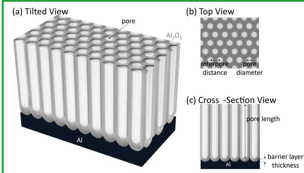
Pore dimensions of anodic aluminum oxide (AAO) are widely tunable by alteration of the anodization process.
