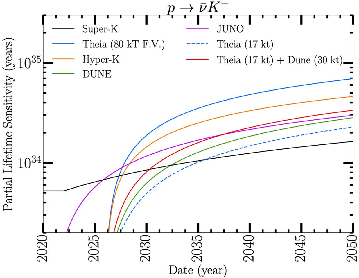
FIG. 19: Sensitivity for  $p \rightarrow \bar{\nu} K^+$  is highest for THEIA, closely followed by the Hyper-K detector, whereas JUNO and DUNE will perform similarly. The inclusion of THEIA in the fourth Dune cavity would provide an enhancement to this mode over the full 40-kt Dune.
