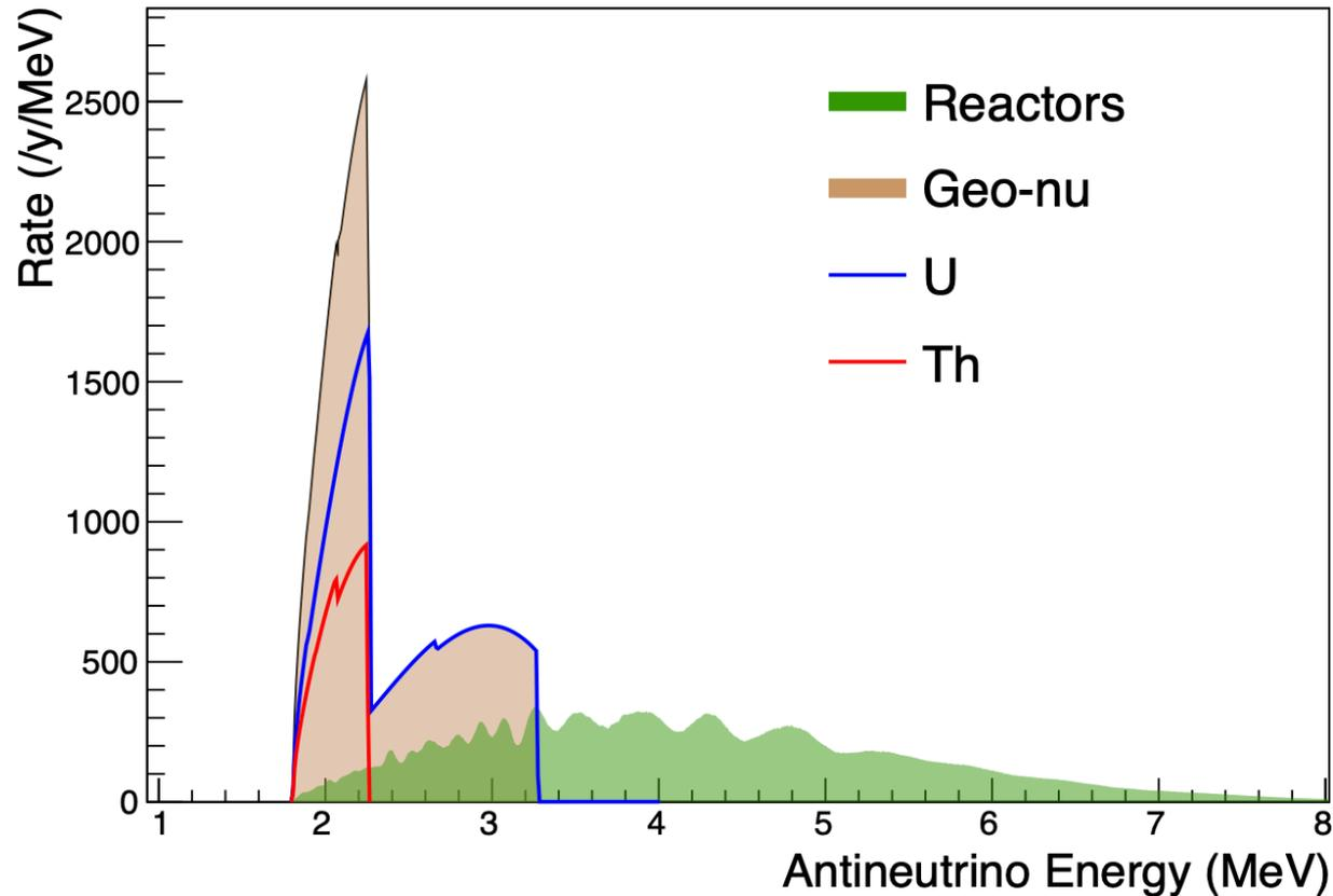
FIG. 15: The detected energy spectrum of the predicted rate of antineutrinos from nuclear power reactors and Earth, assuming a 50 kT water target.
