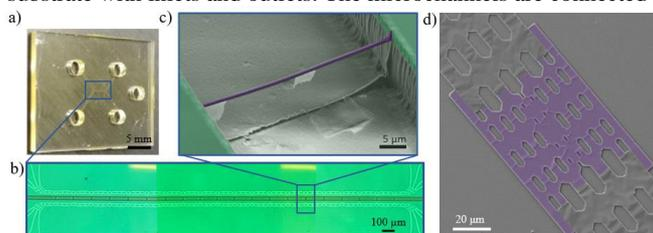
**Figure 2.** (a) These images show a close up of the fluidic structure on the PC substrate. To suspend the nanochannel, a trench is etched into the polymer by RIE (b). (c) shows the suspended nanochannel with a cross section of  $500 \times 500\ \text{nm}$  and a suspended length of  $20\ \mu\text{m}$ . (d) shows a suspended  $\text{Al}_2\text{O}_3$  membrane in a liquid cell.
